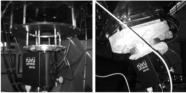
Fig. 10 (Left) EMCCD and barlows. (Right) Fabric covering to reject stray light.
